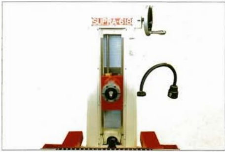
The guideways of the column is hardened & ground to Rockwell C 62 degree. The column is also heavily ribbed.
