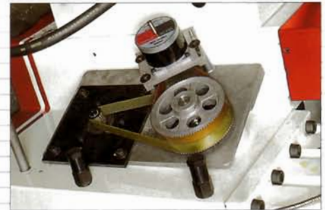
Separated motor controls and downfeed gear panel is a special for 1020 only.
