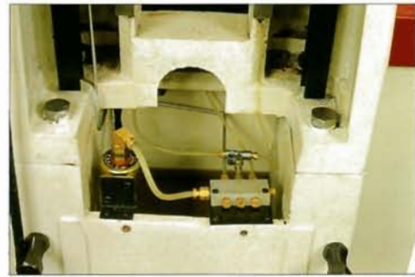
Circular auto-lubrication system. (Model 618 & 1020)
