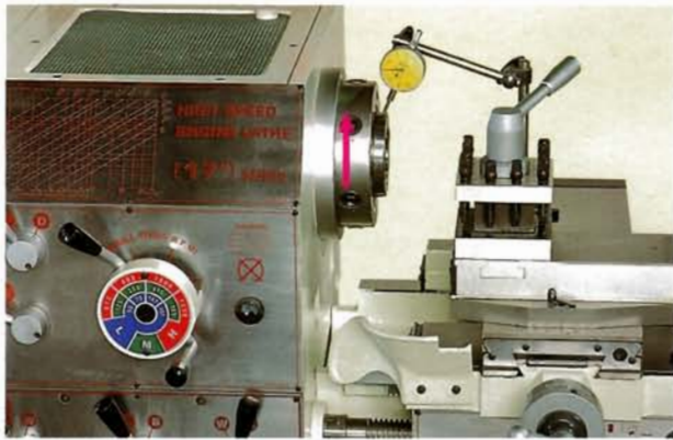
Spindle nose runout A:0.00012" B:0.00024"
