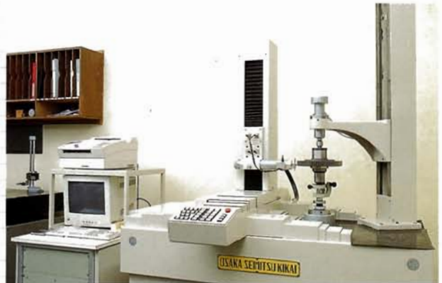
All gears on ACER lathe are tested on the teeth for their final form (within 0.2 micron ). If they are not to the standard, the gear will not be used.
