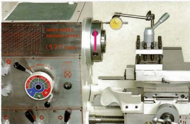
Cam action of spindle A:0.0002" B:0.0004"
