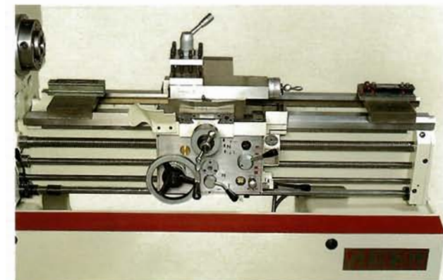
Bed level longitudinal direction A:0.0008/40" B:0.0012/40"
